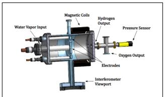
**Fig. 1**. Prototype plasma arc centrifuge under development for experimentation.
